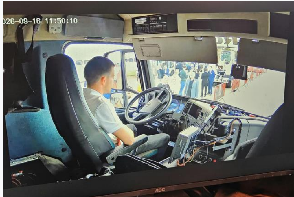
Live cabin view: safety driver on board, tele-operator in control
