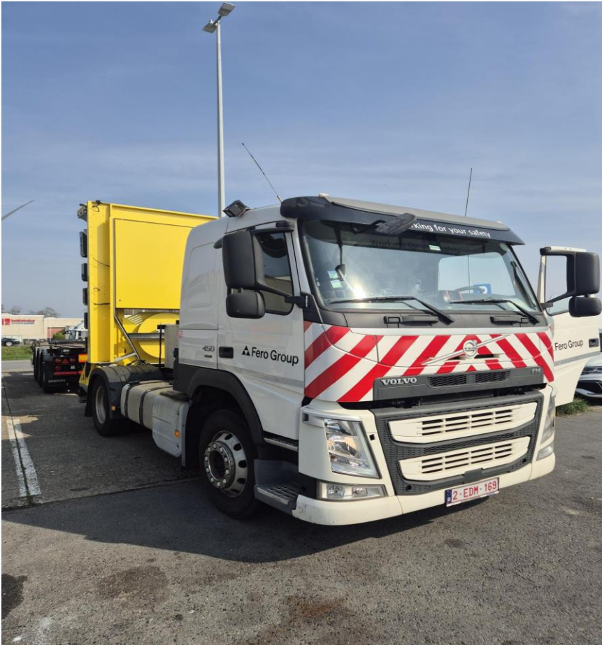
Fero Group — crash absorber equipped with tele-operation kit
